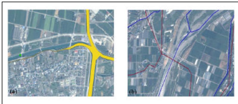
Figure 1. GIS data show errors on an IKONOS image. (a) A river data based on 1 to 2,500 scale maps. (b) A river and road data based on 1 to 25,000 scale maps.
