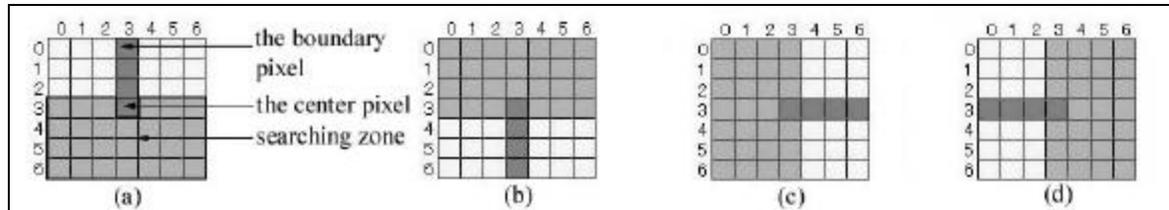
Figure 8. (a) Gradient = 0 or infinite, and y coordinate of center pixel > y coordinate of boundary pixel. (b) Gradient = 0 or infinite, and y coordinate of center pixel < y coordinate of boundary pixel. (c) Gradient = 0 or infinite, and x coordinate of center pixel < x coordinate of boundary pixel. (d) Gradient = 0 or infinite, and y coordinate of center pixel < y coordinate of boundary pixel.
