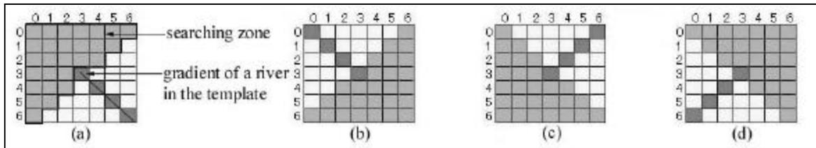
Figure 7. (a) The searching zone, when gradient>0 and x coordinate of center pixel < x coordinate of boundary pixel. (b) Gradient > 0 and x coordinate of center pixel > x coordinate of boundary pixel. (c) Gradient<0 and x coordinate of center pixel < x coordinate of boundary pixel. (d) Gradient<0 and x coordinate of center pixel > x coordinate of boundary pixel.
