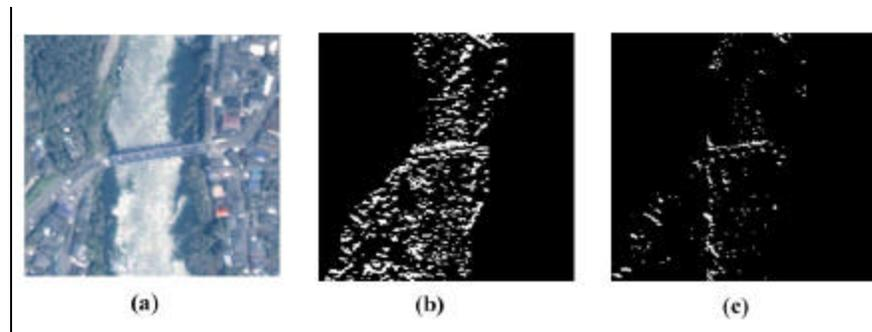
Figure 2. (a) Original image. (b) After applying Line detecting template. (c) After applying Prewitt filter.
