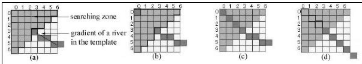
Figure 5. (b) Exist a connecting pixel in the searching zone (c) Connecting (d) Template move to the end of connected line.
