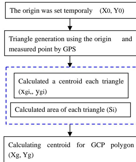
Fig4.1 Flow chart -Calculation method of centroid-
